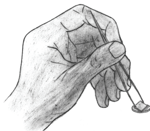
Figure 7.2p Securing Double-sided Tape to the Sample Disk
