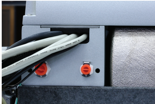
Figure 4.3a Remove the red air and vacuum plugs
