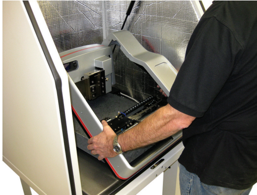
Figure 4.3j Place the cover over the microscope
