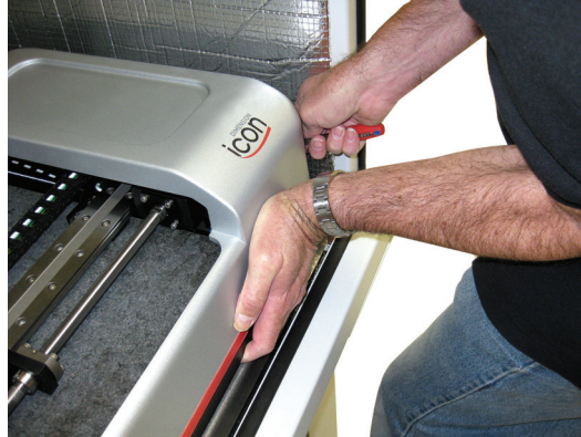
Figure 4.3m Push the front of the cover in to tighten the right front screw.
