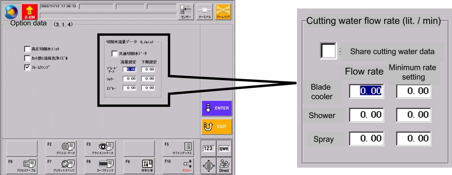
The screenshot displays the 'Option data' screen (3.1.4) with a callout window for 'Cutting water flow rate (lit. / min)'. The main screen shows a table for '切削水流量データ (l./min)' with columns for '流量設定' (Flow rate setting) and '下限設定' (Lower limit setting). The callout window provides a detailed view of these settings for three devices: Blade cooler, Shower, and Spray.
