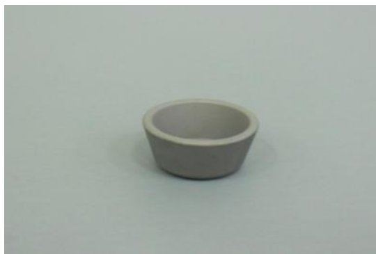
Crucible Liner, 7cc, intermetallic for Telemark
