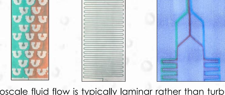
Microscale fluid flow is typically laminar rather than turbulent. Because of this, mixing must be induced through unique channel geometries such as serpentine channels and blockades within the channel. Applications that utilize micro mixing include the preparation of DNA for analysis and detection of chemical content.
