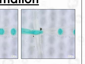
Micro droplets are found in, but not limited to, portable microfluidic devices that perform diagnostic testing, and chemical analyses. They are used to lower cost by reducing residence time, reagent consumption, and power usage. The micro droplet device uses two streams of oil to disperse the water causing it to form water droplets, and shows how changing flow rates can change droplet size and quantity while creating interest in how they are implemented in realworld applications.
