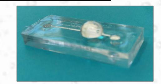
In microfluidic applications such as cytometry (measurement of characteristics of cells), lenses are used to focus and manipulate light to improve device sensitivity. The tunable PDMS lens can achieve various lens radii depending on the amount of liquid pumped into the chamber. These lenses can be placed over cell phone cameras to produce optical zoom up to 37X. This allows one to capture microscope quality images with their cell phones.
