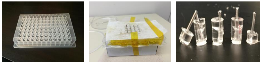
Figure 5.8.2. Well plate pin valve method and produced pins.
