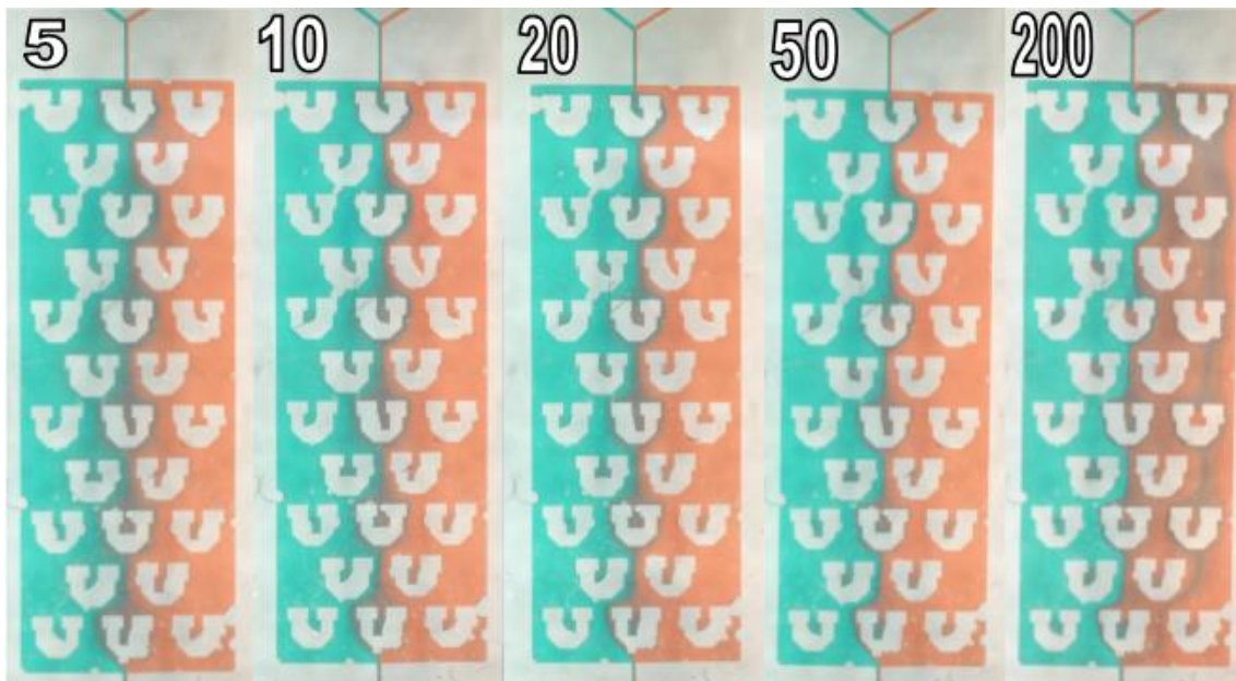
Figure 9.2.8. Mixing results from vertical blockade channel. The numbers represent the flow rate in \mu\text{L}/\text{min} .
