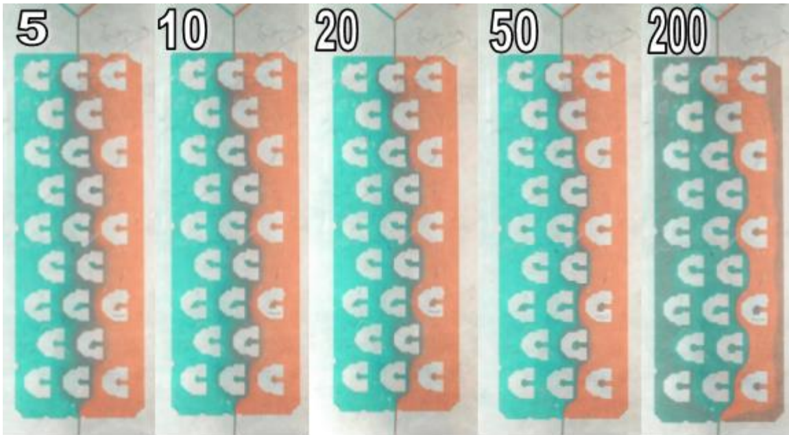
Figure 9.2.7. Mixing results from horizontal blockade channel. The numbers represent the flow rate in \mu\text{L}/\text{min} .
