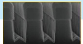
PVD Al deposition on Si - \text{SiO}_2 – the metal layer follows the contour of the etched substrate very well even down into the notches
