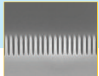
Nanoscale etching by cryo – 50nm lines and spaces – Nanofluidics
