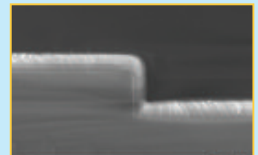
Low stress \text{SiN} film (400nm). Deposition rate 10nm/min, \text{RI} = 2.01 , Stress = <100\text{MPa} . The ICP180 was used for the process.
