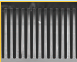
Vertical High AR Bosch Si etch – MEMS
