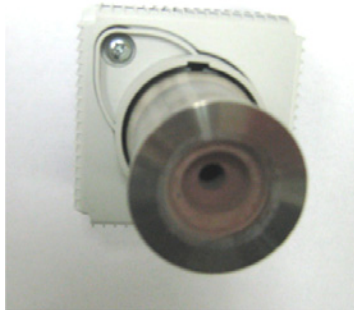
Vacuum gauge with extensive film buildup
