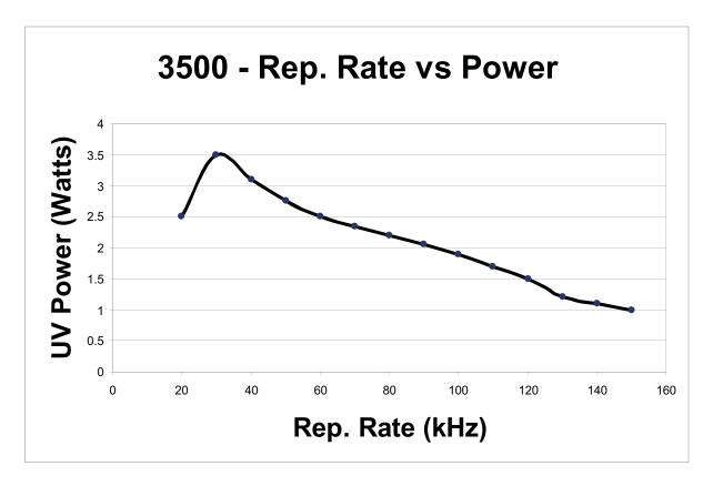
DPSS Lasers Inc. specializes in the production of Diode Pumped, Solid State UV (355nm) laser systems. At the heart of our laser is a Nd:YVO4 (Vanadate) crystal gain medium, which is particularly suited to operate at very high repetition rates. This crystal, in conjunction with our patented (#6,002,695) intra-cavity tripling process, allows DPSS Lasers Inc. to achieve high average power levels at 355nm, while maintaining very high rep rates.
