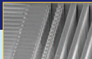
Deep Si feature etch by ICP-RIE cryo process
