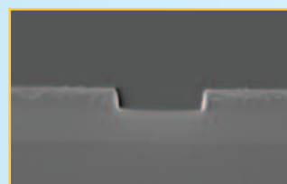
Sub-µm Nb metal RIE (PR mask still in place)
