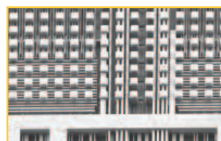
Failure analysis - fast metal layer exposure in the Plasmalab µEtchICP
