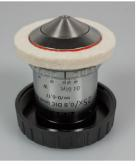
The 25x immersion objective is used for printing medium-sized features. The best surface smoothness is achieved in conjunction with IP-S, hence this objective is recommended for printing micro-optics.
