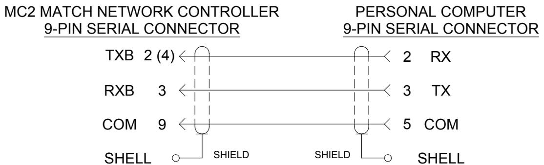
RS-232 Serial Interface Connections to Personal Computer, DB9 Connector
