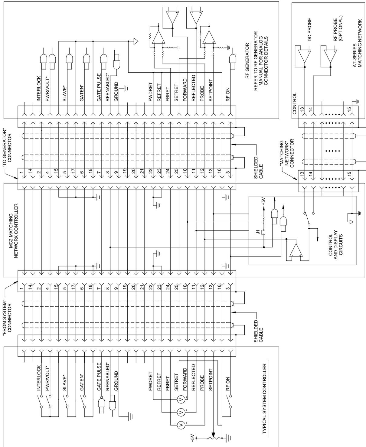
Loop-Thru Connector Interfacing
