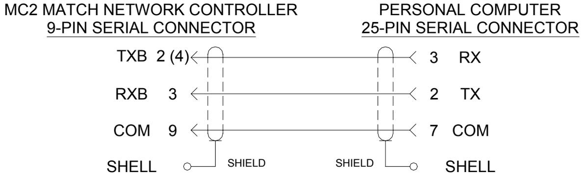
RS-232 Serial Interface Connections to Personal Computer, DB25 Connector
