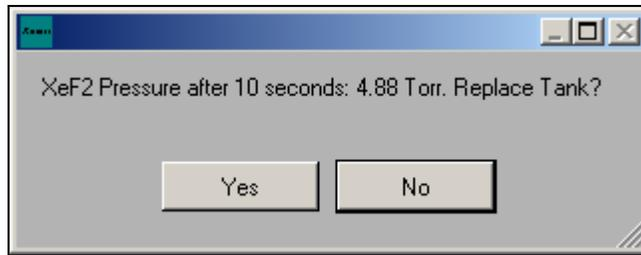
If you have chosen to change the XeF<sub>2</sub> bottle, you will be instructed to close the manual valve on the bottle. Once you have closed the proper bottle's valve, click OK as shown below.
