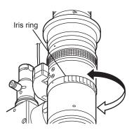
If you reduce the magnification of the lens, iris diaphragm remains OPEN for a while even if you rotate the iris diaphragm ring toward CLOSE. Toward OPEN ×500 Toward CLOSE NOTICE ×300 OPEN ×200 [ OPEN ×100 🗌 OPEN ×50 [ OPEN
