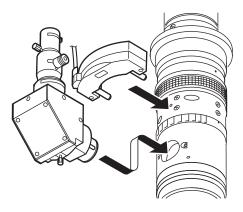
Installing with the VH-S30/VH-S50 free angle observation system
