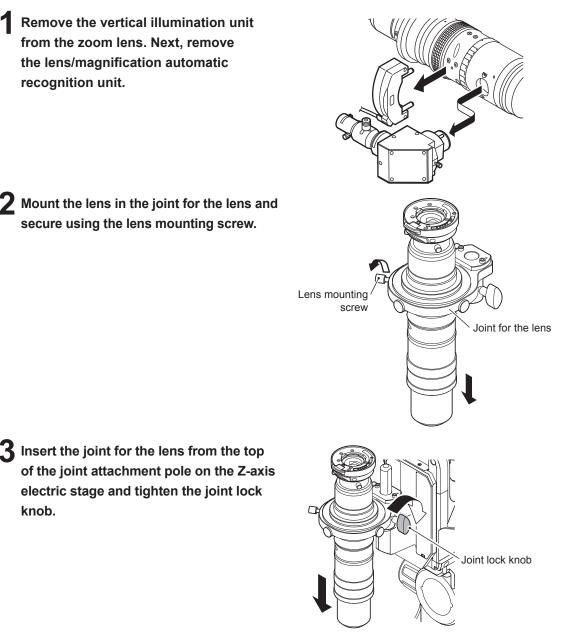
**4** Attach the lens/magnification automatic recognition unit to the zoom lens. Next, attach the vertical illumination unit.
