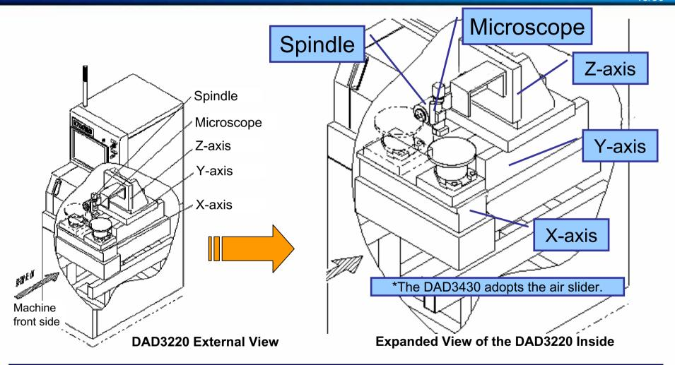
For the DAD3430, a highly accurate air slider is installed to the X-axis. This, together with the high positioning accuracy of the Y-axis, provides high quality processing.
