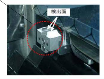
This accessory detects a blade breakage condition and stops the cutting operation immediately, thereby preventing yield loss caused by any damage due to a broken blade in the middle of the cut operation.
