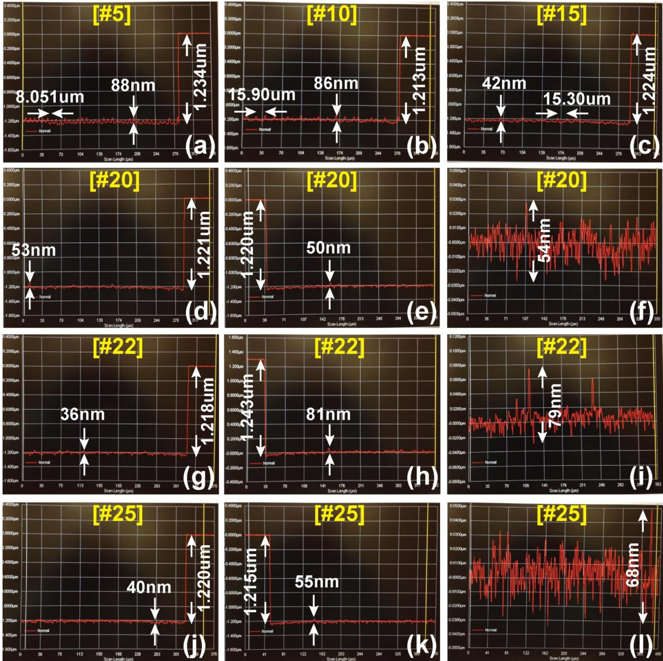
**Figure 3 | Profilometer measurements. (a) – (c) The test exposures numbered before #20. (d) – (f) Measurements of #20. (g) – (i) Measurements of #22. (j) – (l) Measurements of #25. (d) (g) (j) are right edges. (e) (h) (k) are left edges. (f) (i) (l) are central regions. The labeled height difference measurements represent the maximum roughness within the exposure regions.**
