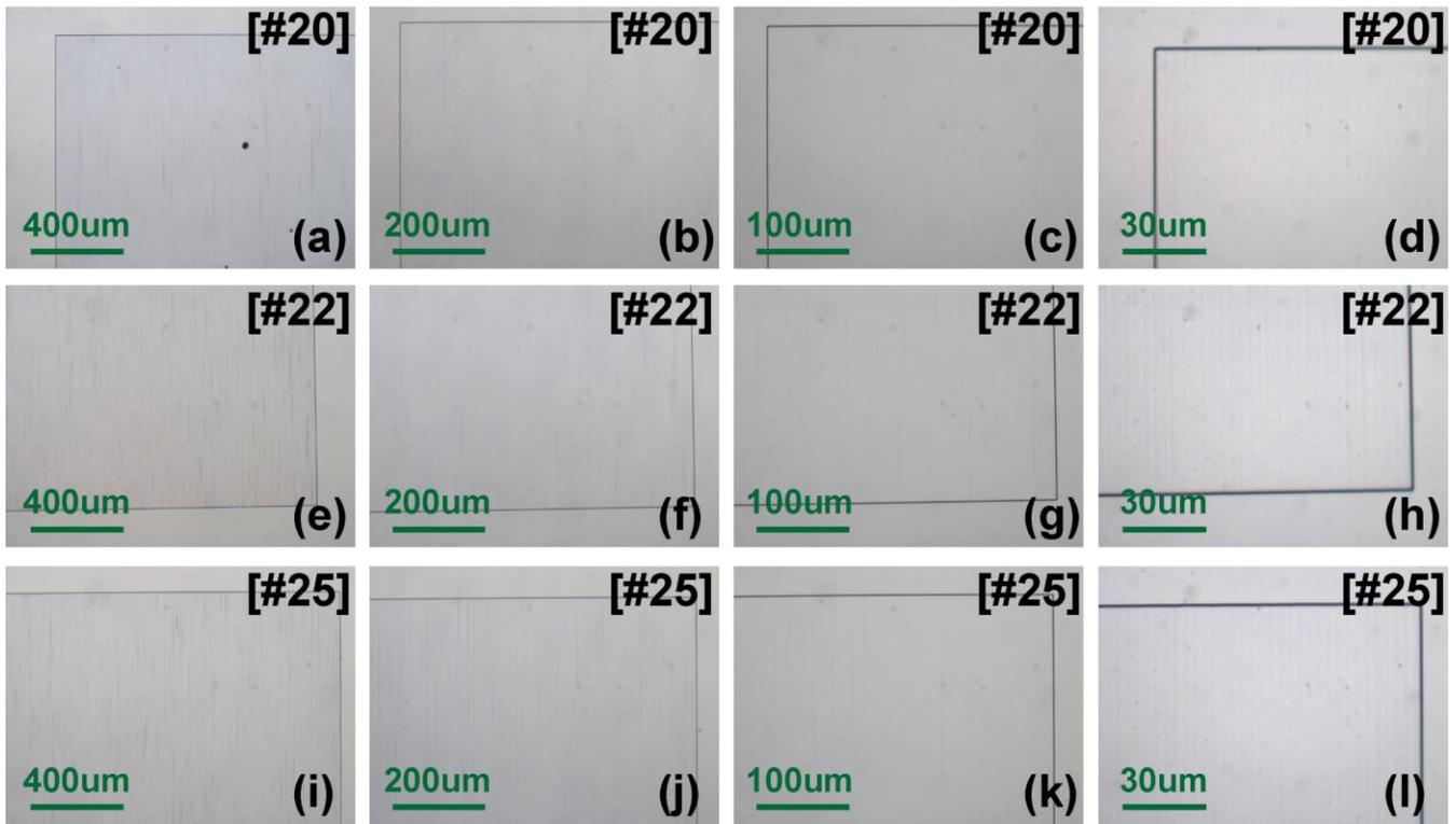
**Figure 2 | Optical microscopic images of the test exposures numbered larger than #20 under front illumination. (a) – (d) #20. (e) – (h) #22. (i) – (l) #25. (a) (e) (i) are 5X magnification. (b) (f) (j) are 10X magnification. (c) (g) (k) are 20X magnification. (d) (h) (l) are 60X magnification.**
