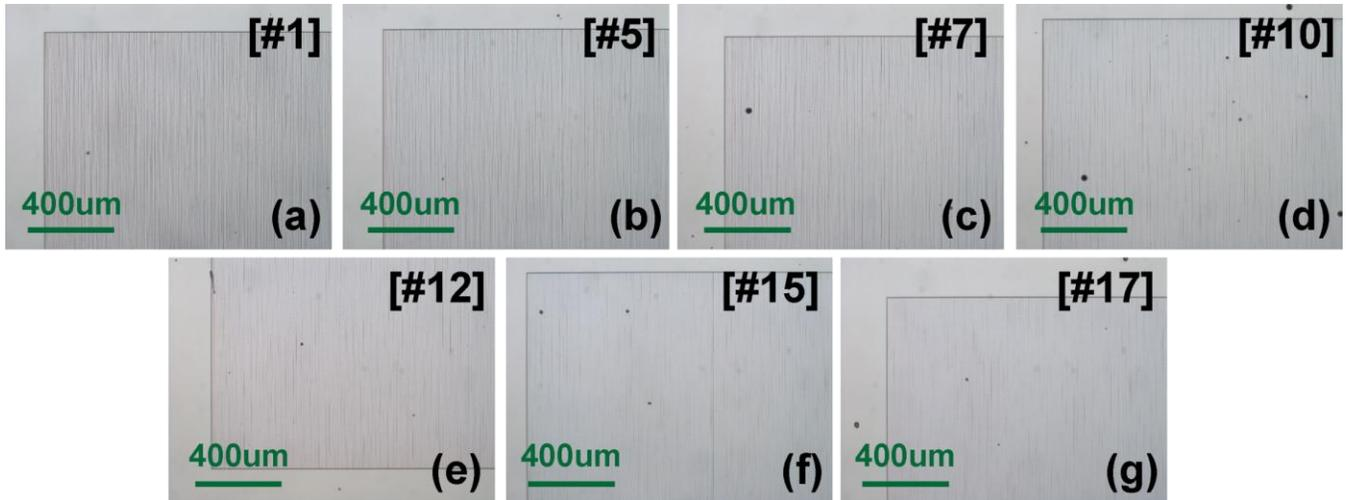
**Figure 1 | Optical microscopic images of the test exposures numbered before #20 on glass substrate under front illumination and 5X magnification.**
