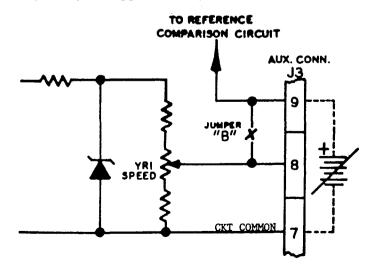
**5.3.1** Open the controller (see Section 9.4.3) and remove jumper "B" located and identified on the main printed circuit board (see Dwg 3-19493).
