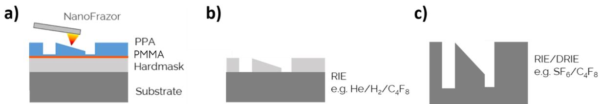
**Figure 26** Process flow for amplified 3D etching. a) 3D topography is patterned in the PPA with the NanoFrazor. b) The pattern is etched first in the underlying hard mask via reactive ion etching. The selectivity of this process need not be high. c) Finally, the pattern from the hard mask is etched into the desired substrate material. The amplification of the pattern depth is mainly determined by the selectivity of this process step.
