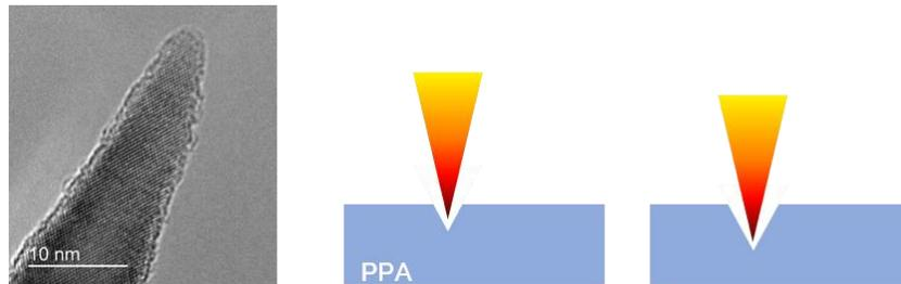
**Figure 12** The NanoFrazor tip is extremely sharp (left) but due to its conical shape the patterning depth influences the maximum resolution achievable (right).
