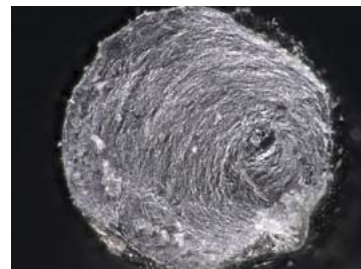
Fractured metal (200x)
