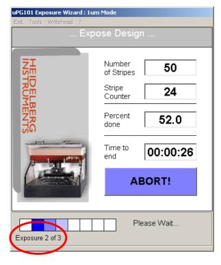
During exposure, progress of multiple exposure job is monitored.
