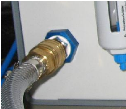
Figure 10: compressed air inlet (supply unit front)
