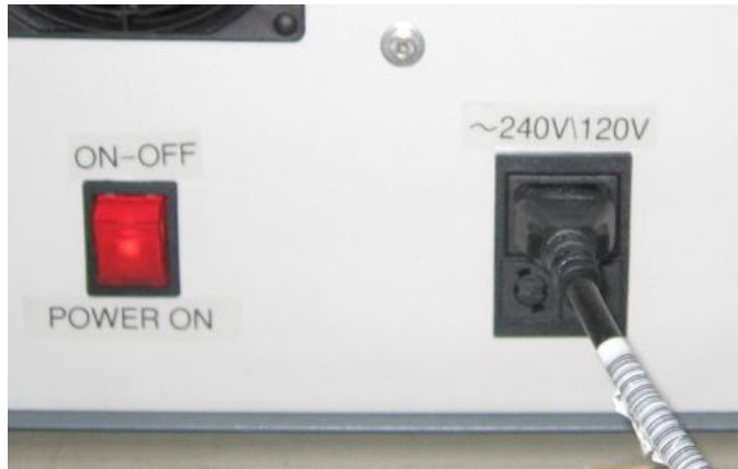
Figure 11: Main power line connection (supply unit back)
