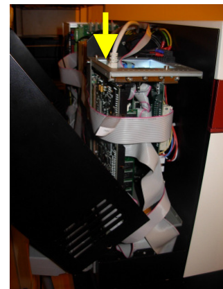
Figure 52: Location of system main board
