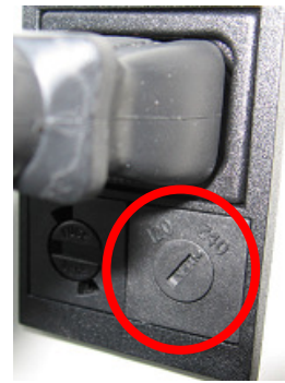
Figure 6: Voltage selection knob
