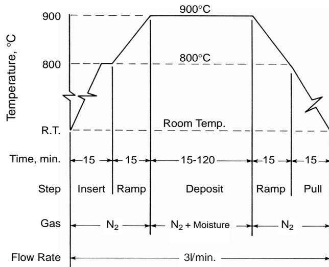
Table II shows maximum moisture levels recommended for depositions made at 850° and 900°C. Since higher levels exceed the rate at which the source can evolve HBO<sub>2</sub> they do not produce thicker glassy films.
