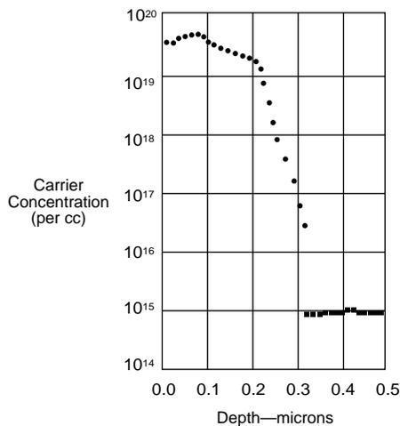
A few selected spreading resistance curves measured on the doped silicon are shown in Figure 5. The silicon slices were first deglazed and then given an 800°C for 20 minutes low temperature oxidation cycle in steam to remove the boron-silicon phase before the dopant concentration profile curves were made.
