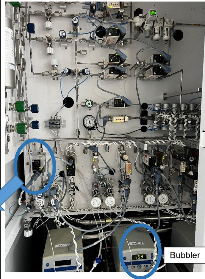
3. **Bubbler to be used is powered on and circulating water.**
